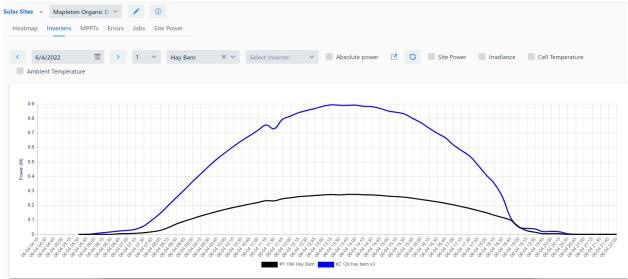
To estimate the current losses on #Y we looked at the total annual output in 2018 for those 2 inverters which was a year with full production because Inverter #Z has been replaced several times. We then contrasted it with the production in 2022.
