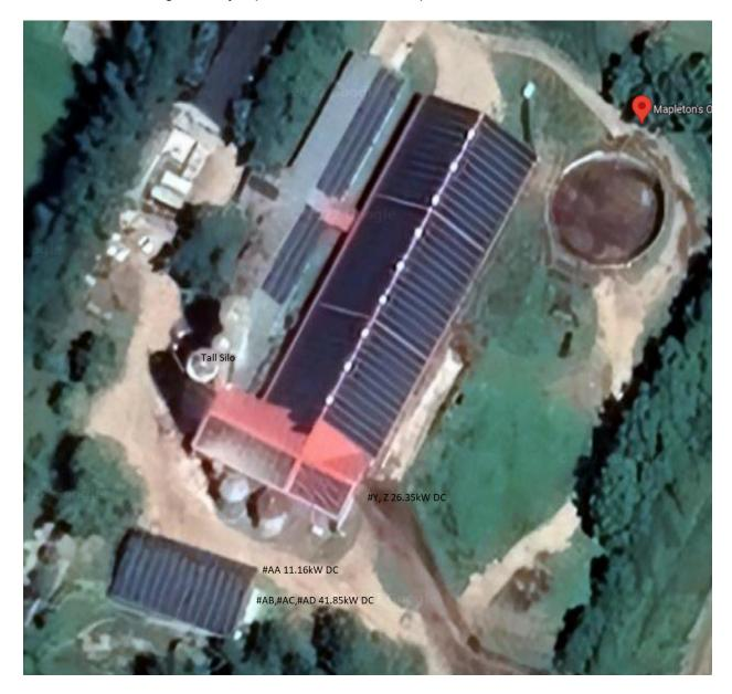
The four inverters we suspect are misconfigured are all on the Driving Shed. The 3 inverters facing south should be the top producers on the site while #AA on the North side would be the worst of the site.
