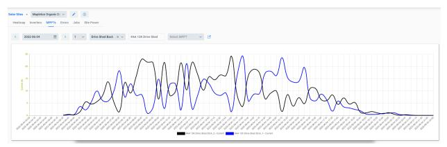
The graphs seem to show that the MPPTs are "fighting" with each other rather than trying to optimize the production. What isn't clear is what is potentially misconfigured. Shown on the next page are the instructions for proper configuration of the inverter which we can then validate on November 10th or could be validated in advance if desired.
