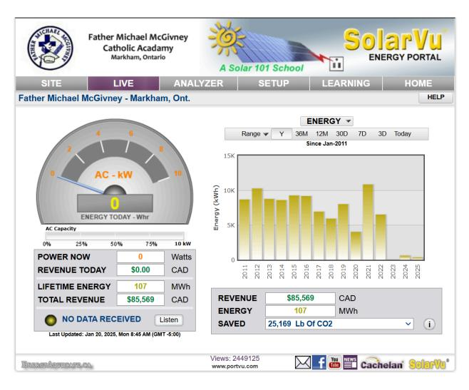
Drop in production may be due to apparent ground faults starting as early as 2011
