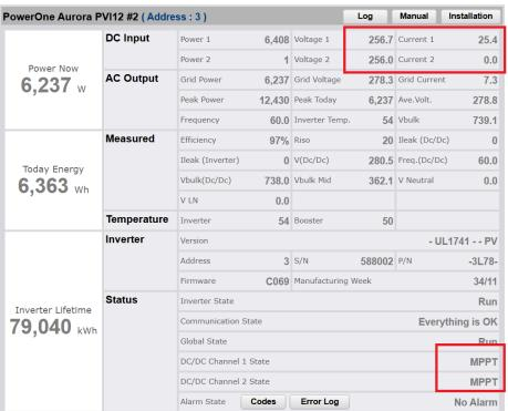
Both MPPTs showing normal voltage and MPPT mode. Only slight power early in morning though on MPPT2
