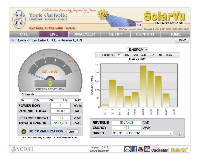
Inverter #1 has startup problems beginning in the spring 2017. Then stops producing on July 9th 2017. Restarts on July 30th, 2020 but at that point won't go past 6.4kW. Based on inverter stats appears to be a replacement inverter so may have been producing for a period of time prior to that.
