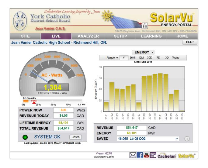
On April 8th 2023 this system appears to have lost production from one of two strings and has been producing at 50% since then. Potentially due to a blown fuse. Loses due to that loss of a string would be approximately \$5,000 since then.
