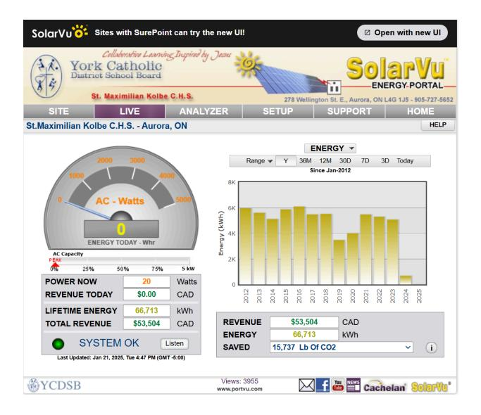
Examining the inverter status at Jan9 2025 at 12:07PM shows the inverter should be able to power up but either has an internal fault or isn't connected to the grid because it won't produce power.
