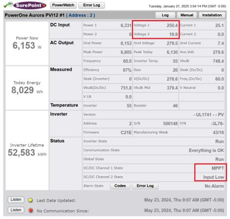
Only MPPT1 appears to have any strings connected. Unlikely at 9:00AM in May that the panels don't have enough indirect sunlight to be showing voltage
